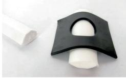
Place the sheet on the arch of the polystyrene molding and wrap the sheet around it, join the edges at the backside, drip with liquid polymer polystyrene. and smooth with a roller.
