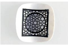
Glue LC Microstencil on the back using instant glue. Glue gradually from one corner to the other. (Use a toothpick to apply the glue. Do not touch with your fingers!)
