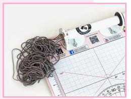
You can make your work easier using LC Tile with LC Vise. Then you won't need any bench clamp. You'll just screw czextruder in mount on the base and by a handle you will easily screw out a snake. It is a great help if you are tired of turning the czextruder by hand or taking out a drill...
