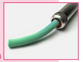
Roll folded skinner blend and put it into the czextruder. Use the first disc with heart shape.
